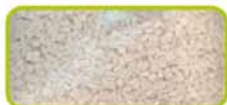
2 2% HBCD board grinded and extruded for recycling + 3% HBCD chiller stab
