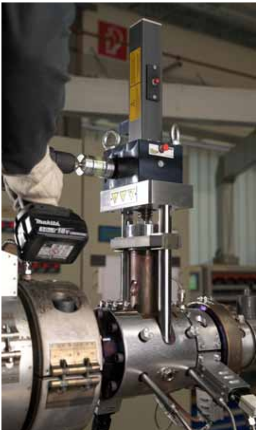
The screen changer is safe to operate manually. To simplify the process, for example, a cordless screwdriver can be used. Photo: W. MÜLLER
