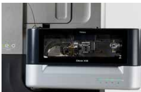
DESI XS and the Xevo MRT Mass Spectrometer for imaging mass spectrometry studies.
