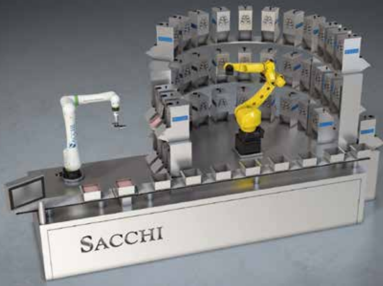
ROBOTIC MICRO AND MINOR INGREDIENTS FLEXIBLE DOSING
